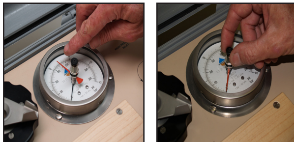
Fig. 31a/b Return the floating needle manually
