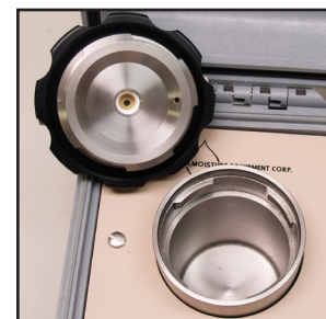
Fig. 3e Specimen holder with safety relief piston
