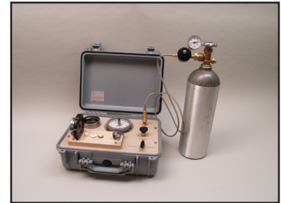
Fig. 1 Portable Plant Water status console
