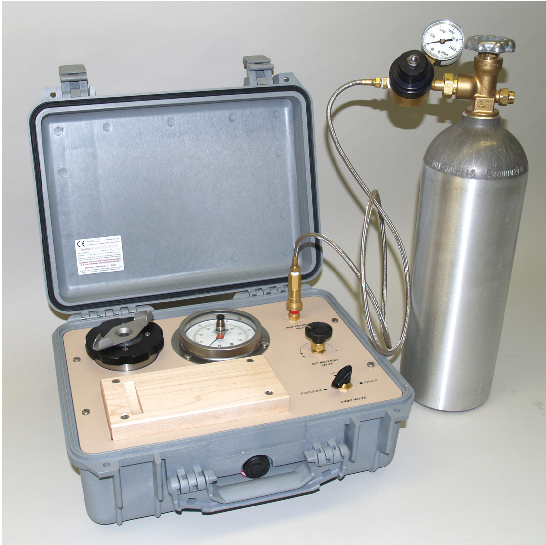
Fig. 1 - Model 3115 Portable Plant Water Console shown with 22 c/f Compressed Gas Cylinder, 3072V22
